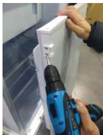
Step 3: remove the screw plug & sliders
