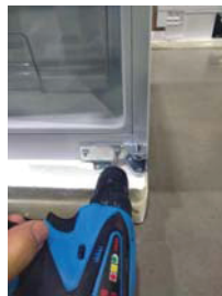
Step 5: remove the lower hinge
