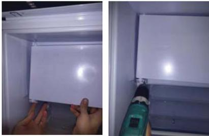
Step 5: insert the door and close, then fix the hinge holder on the left side.
