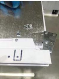
Step 1: remove upper hinge fixing screws and put them aside.
