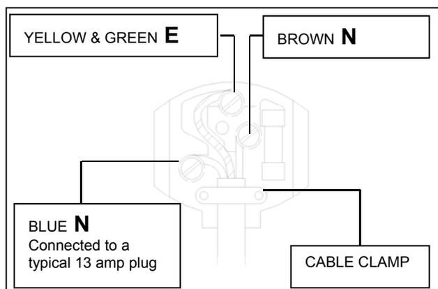
1. The YELLOW & GREEN wire must be connected to the terminal in the plug which is marked with the letter **E**
