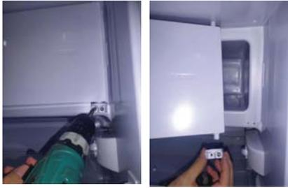
Step 2: remove the inner door fixing screws and put the inner door aside.
