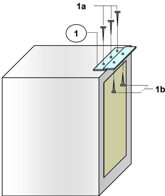
1. Install the top fitting (1) with 3 screws 1a to top of appliance housing.
