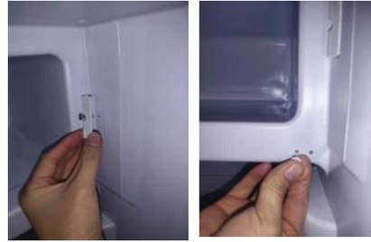
Step 4: fix the inner door block and screw hole plug on the right side.
