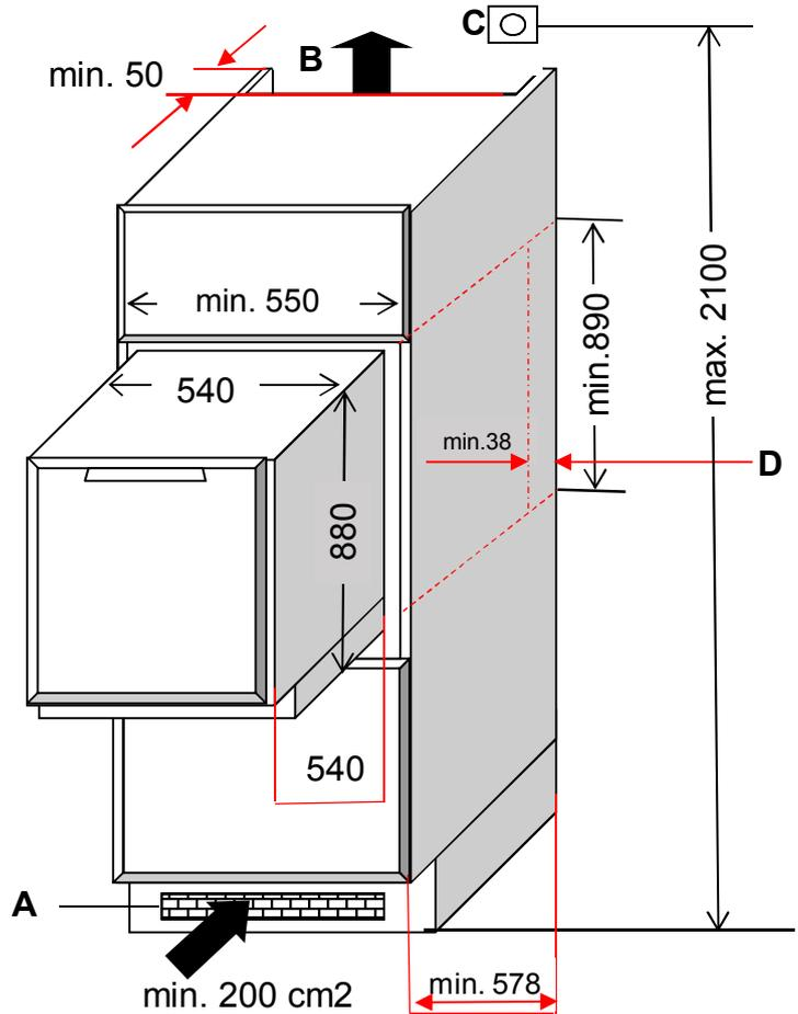
**!** If the mains power connector is no longer accessible after installation of the appliance, an isolator must be fitted on the installation.
